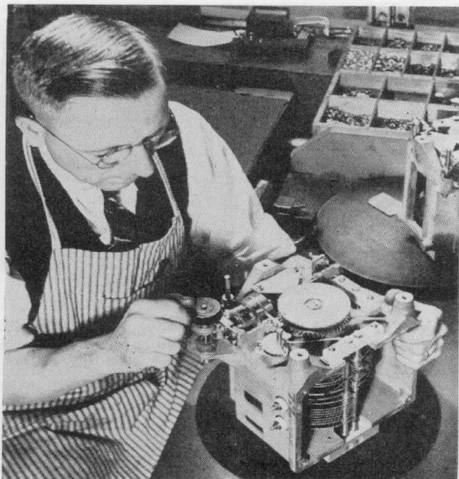
Figure 4. Final adjustments on a Type 622 "bath-tub" capacitor, a special model designed for mechanical stability under extreme conditions.
