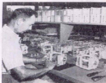
Rotor and stator plates of the Type 1422 Precision Capacitors are individually aligned during assembly.
