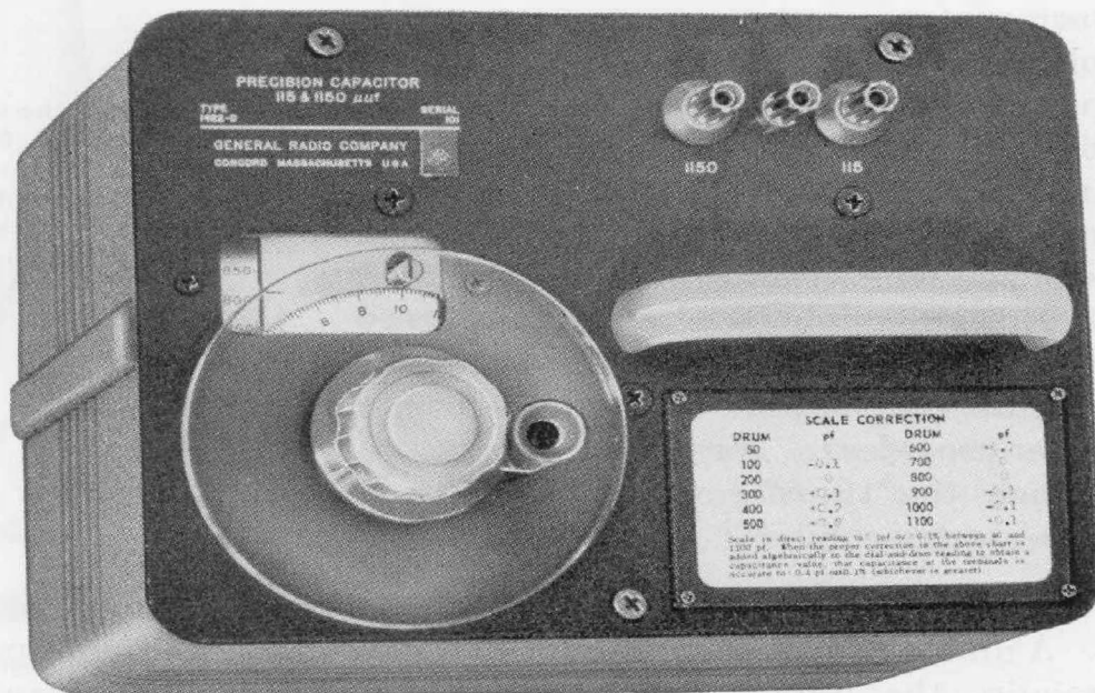
Figure 1. Panel view of the new Type 1422 Precision Capacitor. Note the large, transparent flange on the control knob, which greatly facilitates precise setting.
